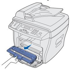
Warning: Do not touch the photoconductor drum located on the bottom of the toner cartridge.
